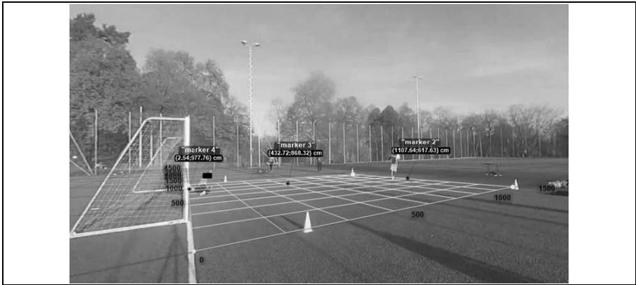
Fig. 8. Fixed image of one kick from the camera behind the goal, represented with the Kinovea motion analysis software showing the marker to assess accuracy.
